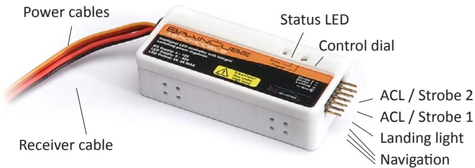
It is important to remember that the controller generates heat during operation, proportional to the number of lights it is running. Mounting it where cooling air can flow over it is required if running more than 10 light modules (2.5A total load).
