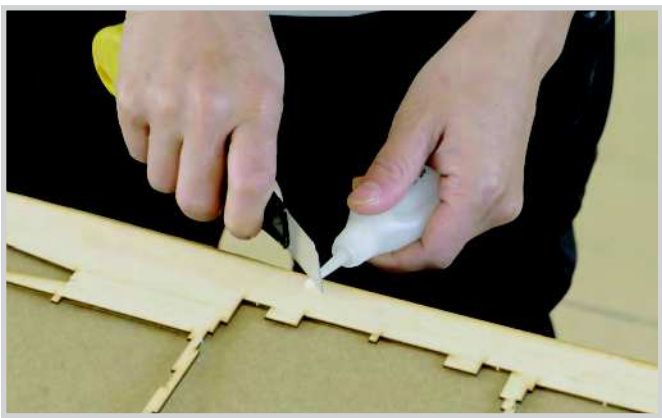
1.11 Cut open CA glue tip for CA application. Make sure opening is not pointing at anyone.
