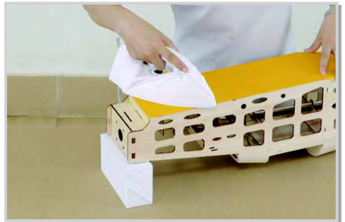
9.3 Tack the covering at corners, this will temporarily fix the position of the covering, and start ironing on the covering. If position is not right, apply heat and peel off the covering and rework. Never try to peel off covering when the covering is cold and adhesive has set, you may pull away wood or separate the color layer. Always heat up the covering to melt the adhesive before peeling.
