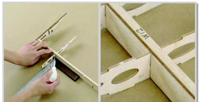
5.3 Glue in W12A/W13 assembly perpendicularly to W9, note that W9 is the wing tip end and should be perpendicular to W12A/W13.
