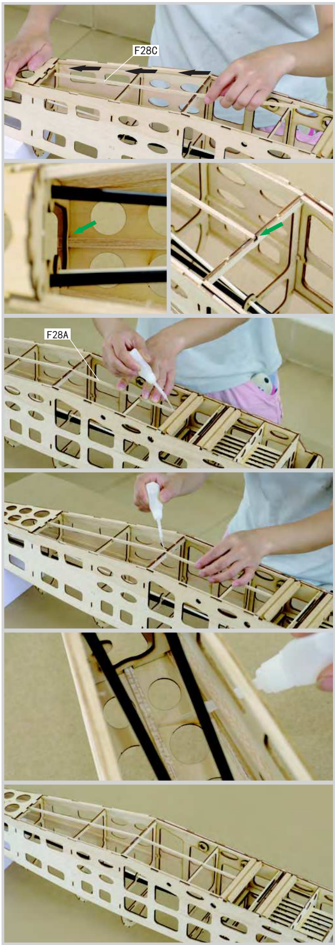
3.2 Insert F28C into tail section of fuselage, note that it should pass through the notch of F10, and share the notch of F7 with F28A, apply glue to fix in position.
