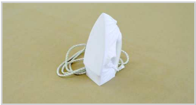
9.1 Cover iron with cotton cloth to eliminate scratch and better temperature distribution. A hobby grade sealing iron with cover sock is recommended for better handling.
