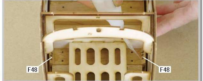
3.6 Flip over fuselage and glue in reinforcement bars F45, F45A, F46, F47 and F48.
