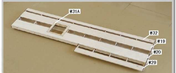
6.8 Flip over wing with bottom up, glue in W31A, W32, W19, W20, W29. Align the hole on W19 with the blind nut hole for wing strut installation. Apply CA to glue all surfaces in contact.
