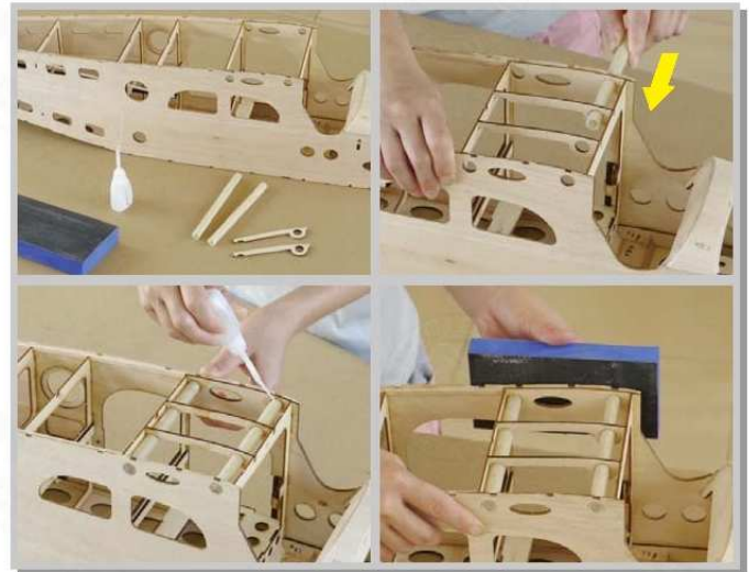
4.1 Insert wing tube sleeves into fuselage. Apply glue to fix them in position. When cured use sand paper to grind down sleeves to flush with fuselage side panels.
