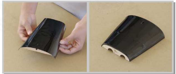
11.10 Cover the battery hatch. Cut a slit on the covering for the latch knob before ironing.
