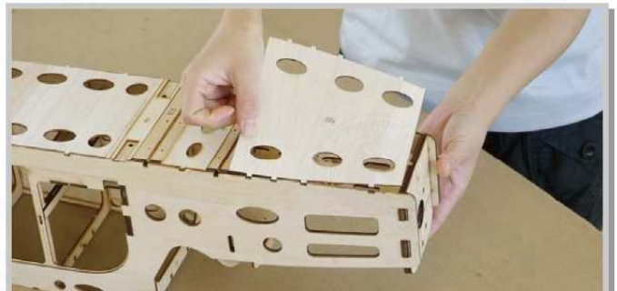
3.6 Flip over fuselage and glue in reinforcement bars F45, F45A, F46, F47 and F48.
