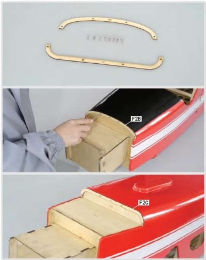
6.13 Use PWA2x8 mm screw to fix F2B and F2C.
