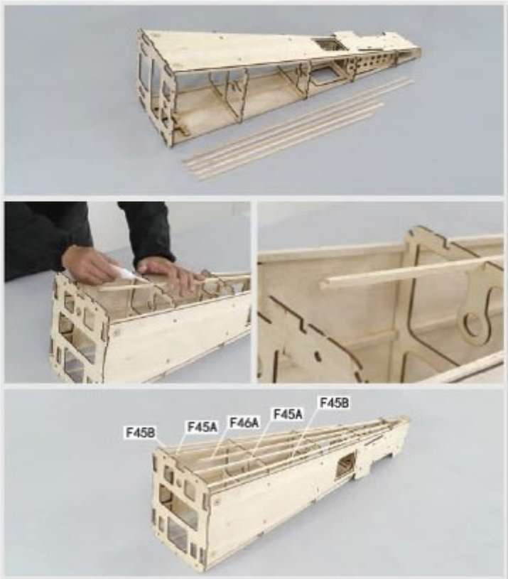
4.7 Flip over tail section and glue in F45A, F45B and F46A. Place F46A with slots facing outwards.
