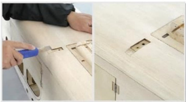
4.32 Cut out landing gear slot.
