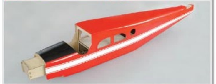
6.12 Install cowling and tail section to the fuselage. With reference to cowling trimming pattern, add on fuselage side panel trimming. After trimming is done, cut trimmings at junctions to free door and servo mount.
