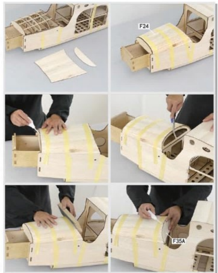
4.29 Apply slow curing glue to surfaces in contact with F24. Apply moisture to outer 6 cm portion of F24 then put on top of frame. Use tape to hold F24 in position. When cured remove rough surface by knife and sand paper. Glue in F35A.
