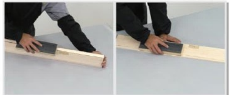
1.32 Remove rough edges at both ends with sand paper, then glue W27 in place.
