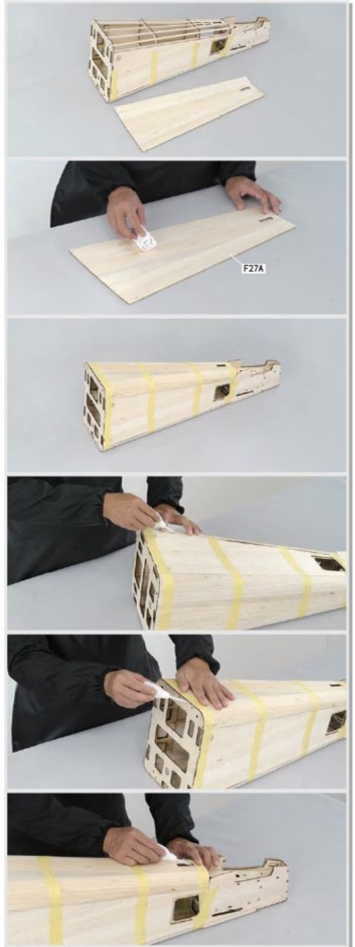
4.11 Place tail section upright, repeat same procedure as 4.9 to glue F27A in place.
