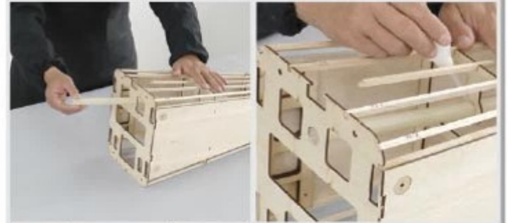
4.5 Put tail section upright and glue in F70. Make sure latches are fully inserted into slots when applying glue.
