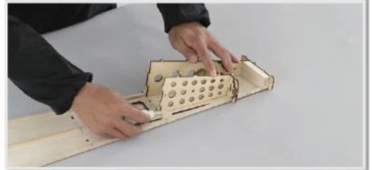
4.3 Insert F13 and F72 into side panel. Apply glue when both F13 and F72 are in position.
