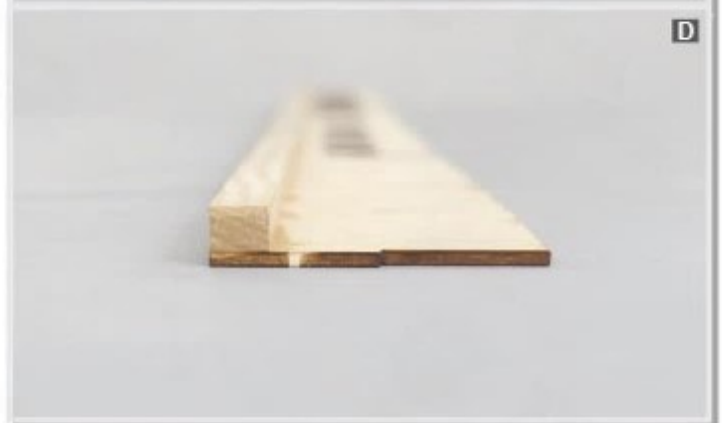
1.3 Glue and join W15 to W15A, W16 to W16A. Glue wider side of W15/W15A to W16/W16A. Place the W15/W15A joint as far away as possible from the W16/W16A joint.
