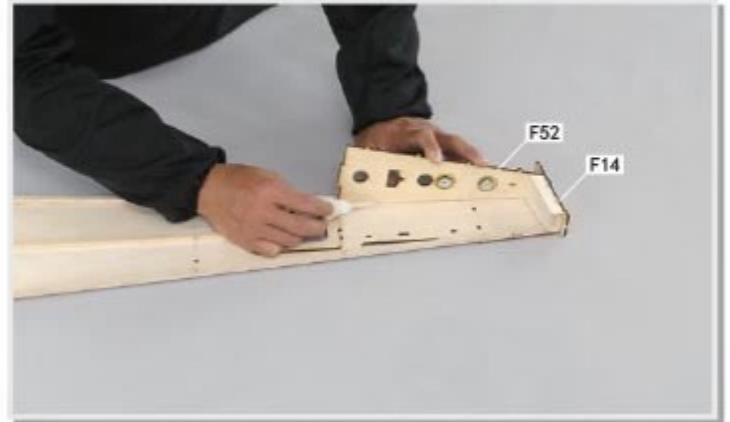
4.2 Glue in F14 and F52, make sure all the latches are inside corresponding slots.
