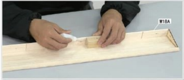
1.29 Glue W25A in place at both ends. Glue W31 to W35A opening, then glue W18A in place. Make sure W31 tapers towards the trailing edge.
