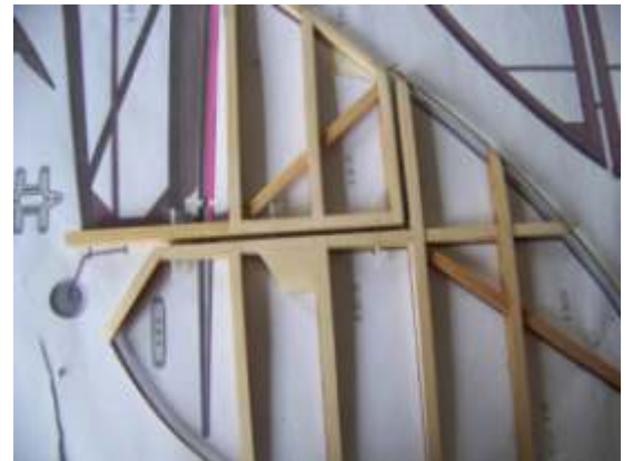
(8) Bore and install the needle hinges. The vertical fin is finished.
