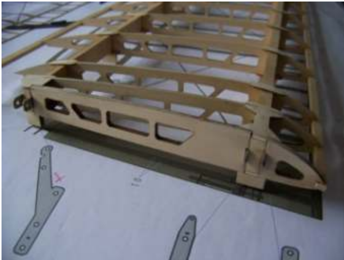
(8) Accurately make 2pcs D1 ribs coincident with resin glue ,Joint it on the wing.
