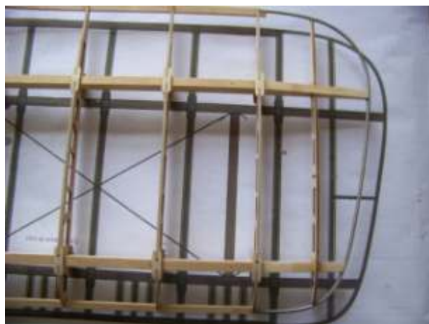
(2) Bend the 4mm stainless steel tube according to the installation drawing, then glue to the wing. Suggest using fiber cloth to strengthen the sticking-joint.
