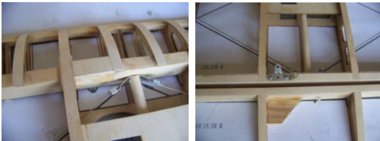
(16) Install the appropriate wood block on the mount of wing strut, and smooth it, then install the metal parts like the pictures.
