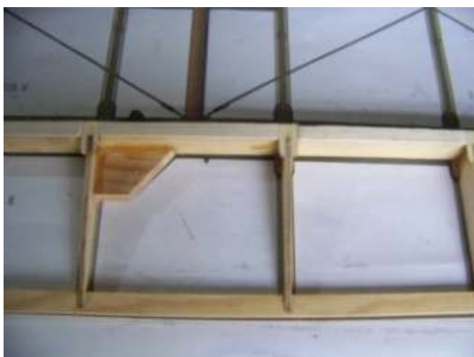
(14) Joint the strengthening plate for servo horn.
