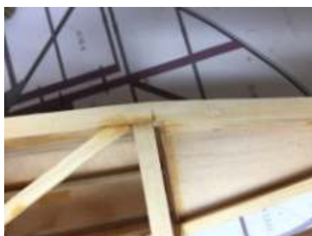
(13) Make a small cut for bending the battens easily. Then joint A23*2 & A24 , and the diagonal pillars, strengthening plates like the pictures.
