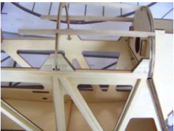
(7) Sanding the strengthening plates.
