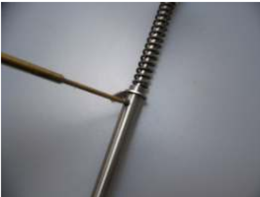
(3) Joint the spring & sliding sleeve, and lock with each end of nuts, then insert it to steel tube and the connection, keep the shaft movable.
