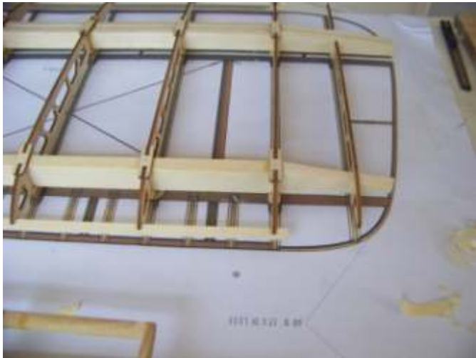
(6) Install the aileron girder, and insert&glue the strengthening plates.
