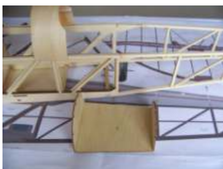
(10) Joint and glue A17,A18,A19(cabin),Then glue the part on the fuselage like the pictures.
