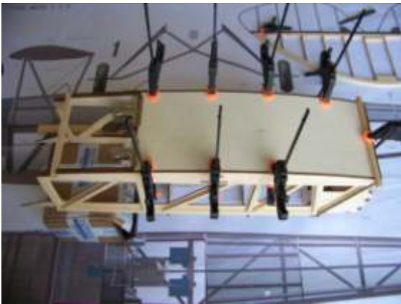
(4) Glue the bottom board A37.
