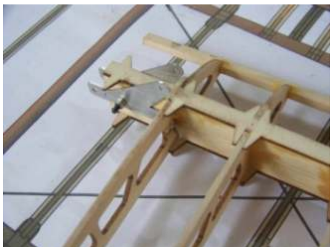
(9) Mark the place of center line and then bore 3mm holes according to the holes of metal parts. And install the metal parts.
