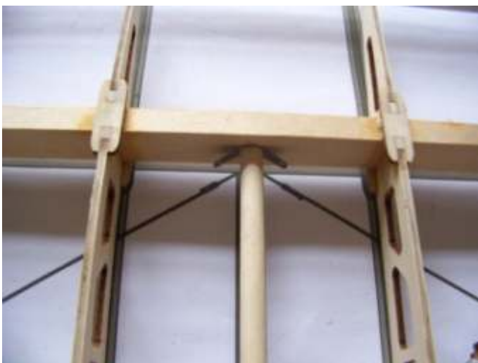
(10) Fix the 8mm wood bars and metal parts with self-tapping screws.
