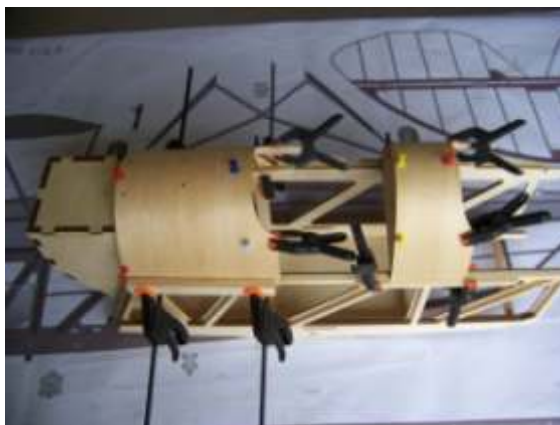
(8) Glue the top cover board. Then glue A10*2,A11*2,A15*2,A16*2 according to the installation drawing.
