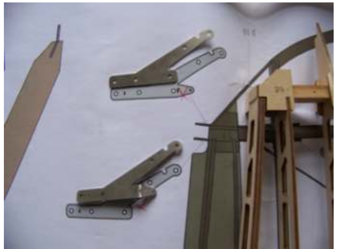
(4) Notice: the right side of the metal parts is counter to the installation drawing. Sorry for that and we will correct the drawing in next batch production.
