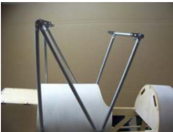
Supporting for the fuel tank.
