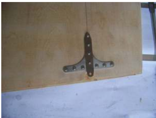
(17) Install the wing mounting metal parts with self-tapping screws.
