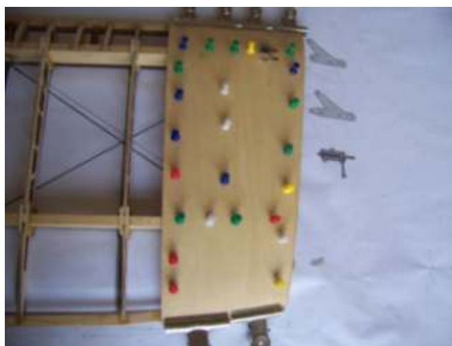
(13) Glue 1mm plywood board (up and down).
