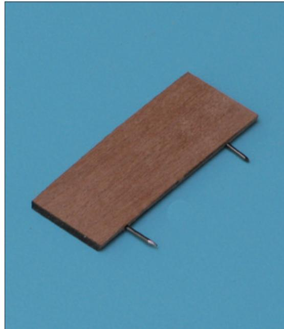
◀ Cut out all of the channels from their 2mm wood sheet (94- 97). Drill a hole at each inner edge of each channel as shown. Cut off the heads of the pins and insert them into the holes. This is to ensure that each channel is very securely in place on the hull sides, as they will have to take a lot of strain from the rigging.
