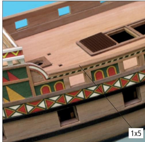
▲ After 198 is in place, add the main 1x5 mm strip in place as shown.
