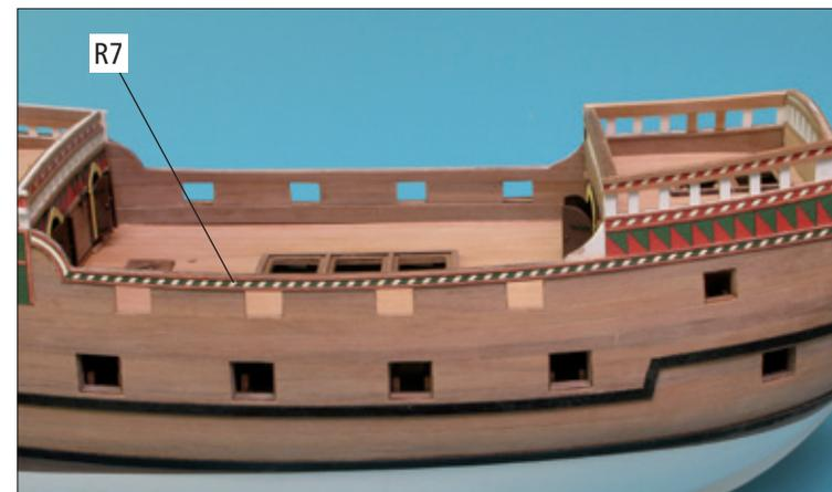
▲ Cut out and apply both R7 and L7 directly below the mid-deck outer bulwarks and all the way to the end of the forecastle as shown. Because of the length and narrowness of these two parts, take extra care when fitting into position.
