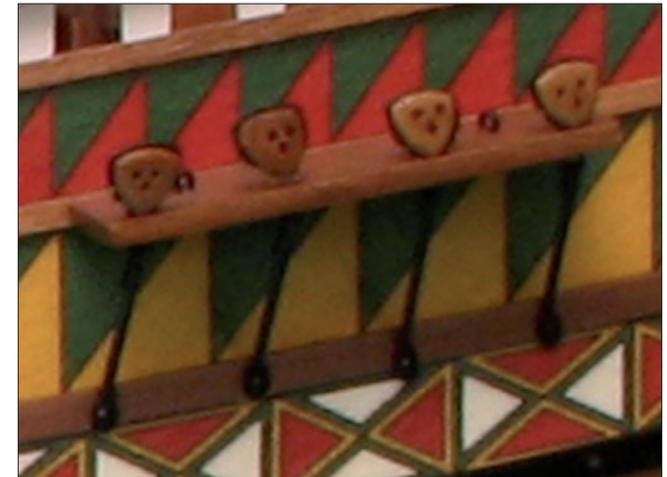
▲ Mizzen and bonaventure channel detail - 1:64 scale. use this drawing for obtaining the correct angles of the chainplates. (All 5 mm deadeyes).
