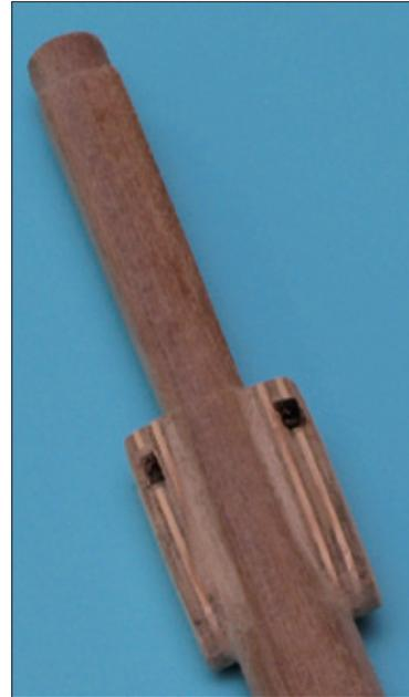
Using the main plans, make up the mast as shown and then add the cheek assemblies from parts 185-187. Glue 186 and 187 to the inside surface of 185, so that there is a gap near the top for the main jeer rope to reeve through. Then add the other 185 pattern to enclose the slot at its sides. Glue the completed cheek assembly into position on the main mast. If there are any gaps between the cheeks and mast, fill them with wood filler and sand smooth.
