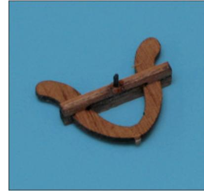
◀ Make up the eight sets of staghorn cleats as shown. Drill a hole to the back of the crossbeam and insert a headless pin to help secure the assembly once in place.
