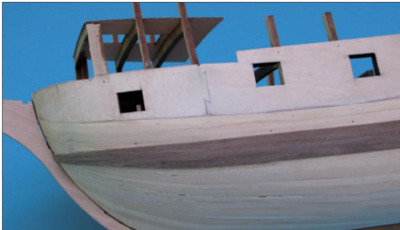
▲ The first three planks (per side) laid using superglue to avoid pin holes.
