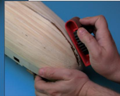
Finally sand the first planking until a smooth surface for the second planking is attained. Sand the whole hull that has been planked with a coarse grade abrasive paper, followed by medium grade. This will entail about an hours work. If possible, sand the hull in a well-ventilated area, ideally in an open space as the dust particles could present both a fire and health hazard. The use of light duty gloves is also recommended to reduce any risk of blisters from sanding.
