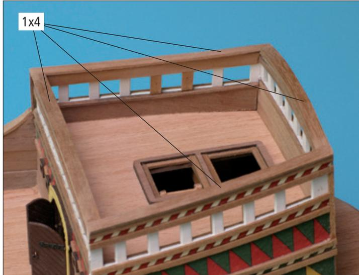
Measure and cut to the correct length the mid bulwark capping from 1x5 mm strip. The curved capping is found on the 5 mm hardwood laser cut sheet (Parts 198 & 199).
