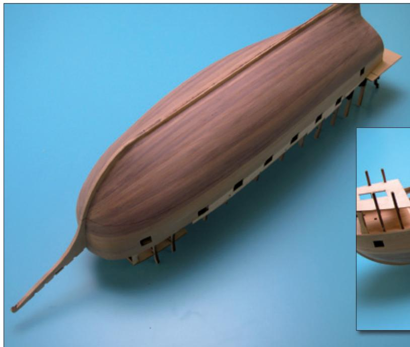
Use a waterline marker to mark out the waterline as shown. Use the full size hull plan to determine the correct height of the waterline from the keel.
