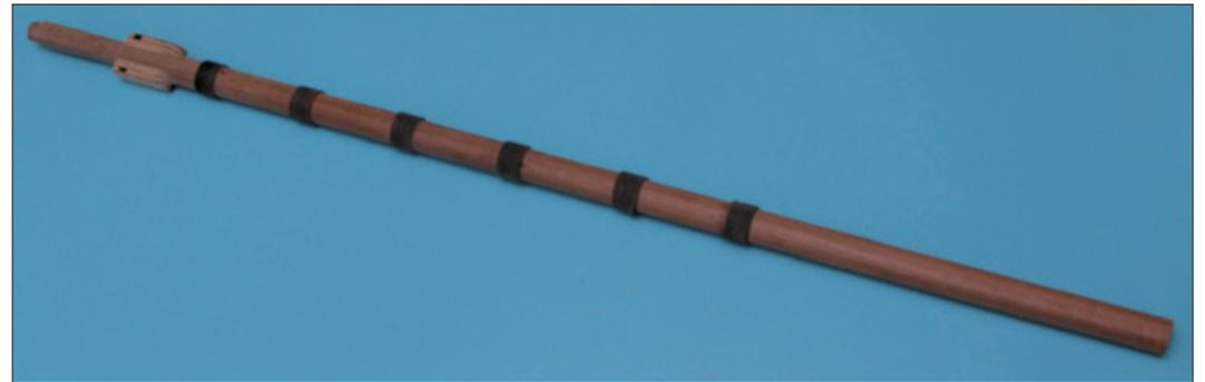
Paint the area between the lower mast cheeks and the lower mast cap black, as shown. (Same for all masts).
