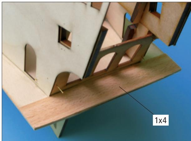
◀ Start the gallery planking at the back, as shown using 1x4 mm Tanganica strip. Be very careful not to get glue on parts 51 and 118, as they have to be removed once the outer gallery planking is complete.
