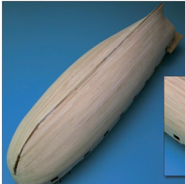
First planking complete. If you have any large gaps in-between planks, fill them with wood filler to ensure the second planking has maximum contact with the surface it is glued to.
