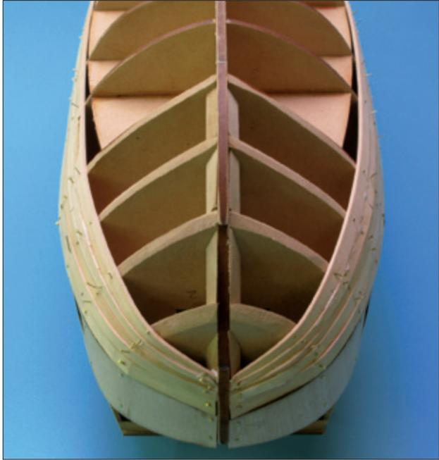
▲ Planking progress fore and aft. Do not worry if you see the planks less than flat at the extremes, this is normal and will be sanded smooth once planking is complete.
