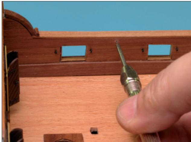
▲ Drill a 1mm hole into the staghorn cleat position on the inside of the bulwarks as shown.
