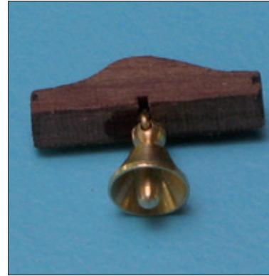
▲ Drill a small hole in the centre of the notch in part 191 and glue and insert the eyelet (attached to the bell) into the hole.
