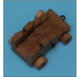
▲ Drill a 0.8 mm hole (or 1 mm if you haven't a drill that small) in each carriage side and on the back as shown.
