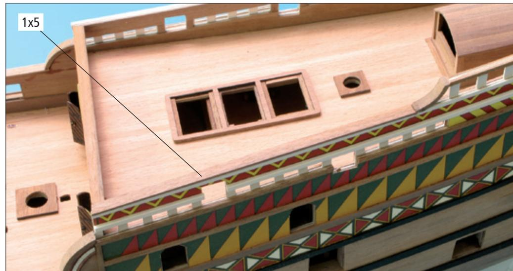
▲ Cut to length the quarterdeck bulwark capping (1x5 mm wood strip), and glue in place as shown.
