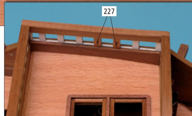
Drill and glue an eyelet (227 - from the photo etched sheet and painted black) into each end of the inner gunport openings on the main bulwark, quarterdeck and forecastle, as shown.
