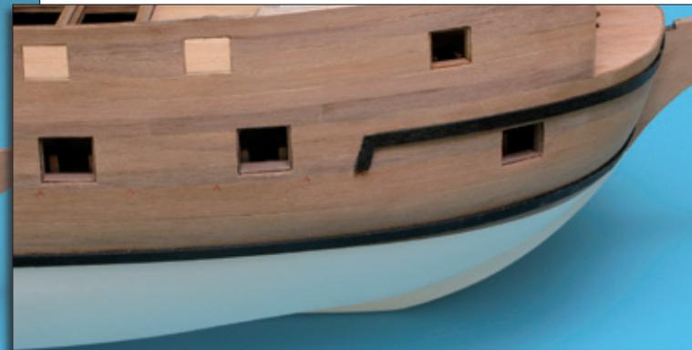
◀ Before adding the main strip, mark out and cut to size the angled wale that connects the two stepped wales together using 1x5 mm wood strip.
