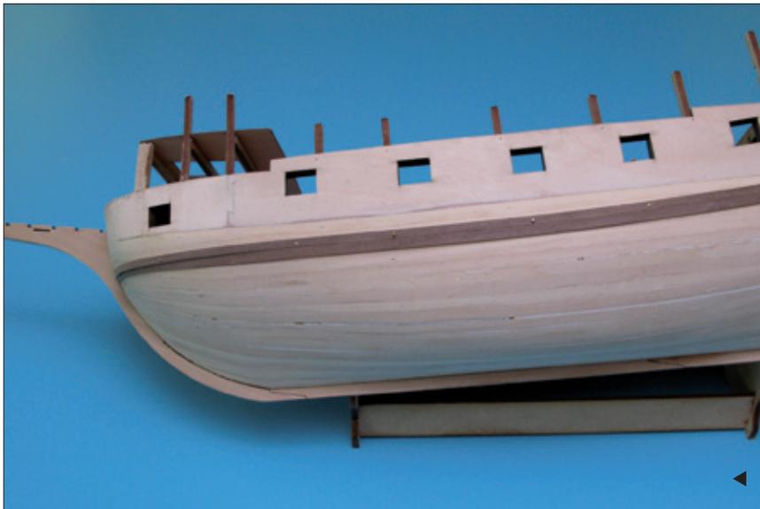
◀ First plank glued in place. This is the most important to get right, as the shape will dictate the run of the planking above the waterline, and the upper wales.
